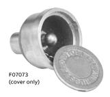
— Aerospace/industrial static ground devices Static grounding receptacles are used in airport and aerospace installations worldwide during fueling, testing and maintenance procedures. Normal mounting is concrete/tarmac floor inset, threaded onto copper ground rod.
