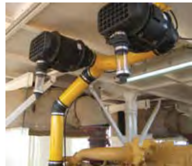
The addition of Dust Dumpa tube extensions to this double PSD air cleaner application provided extended filter life on this Australian geothermal drill rig.
