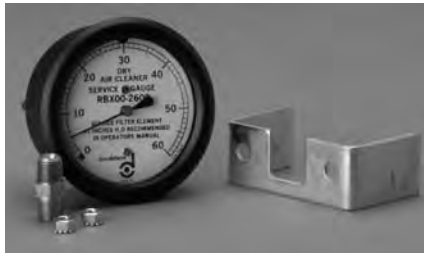
Gauge Part No. X002700 Restriction Limit: 60" H 2 O/ 15 kPa Kit includes restriction tap fitting (P112257), nuts, mounting bracket and installation instructions.
