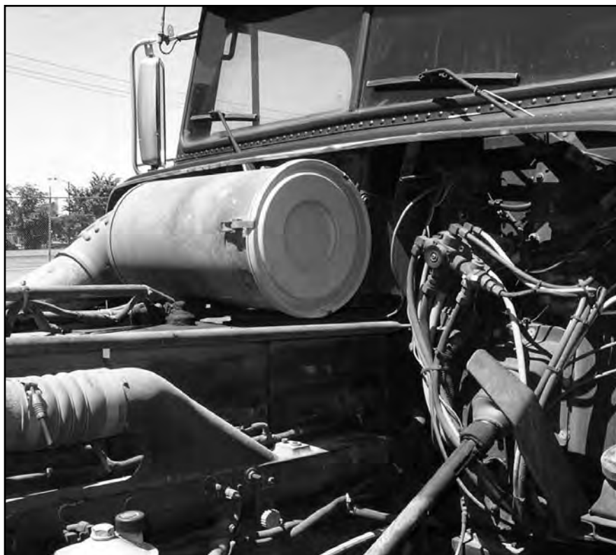
This ECG Konepac model is mounted to the fire-wall on this on-highway truck. The latched service cover allows for easy access to the filter for change out.
