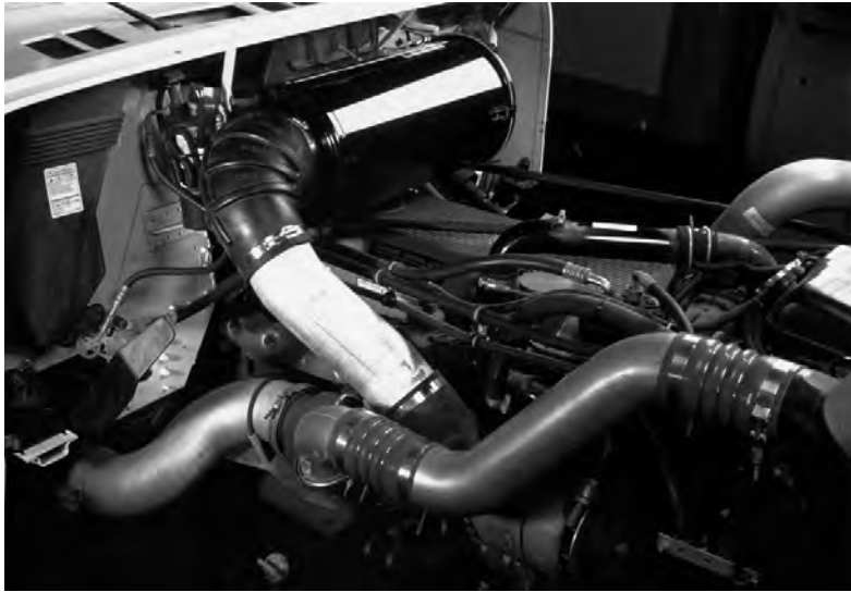
Picture of A112018 air cleaner with service cover on the opposite end of the inlet.
