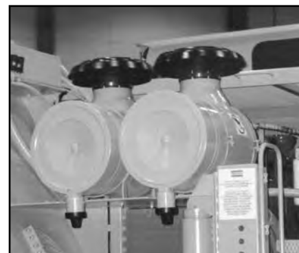
FVG air cleaners are used in tandem on this underground mining equipment to double the airflow throughput to the engine.
