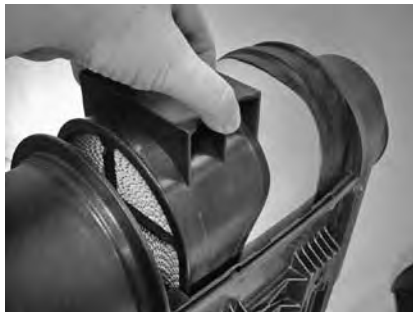
The filter on the side service access models can be easily removed with the built-in grab handle.
