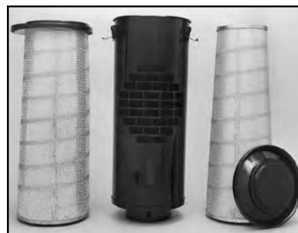
ECG Konepac I with Perforated Inlet - an alternative to disposable style housings. You'll get the economy of replacing the filter instead of the entire unit each time. The perforated inlet on the side of this G112417 housing (middle) is the same as the disposable's, so conversion is direct and easy. Left: Extended service filter. Right: Filter designed for scheduled maintenance.
