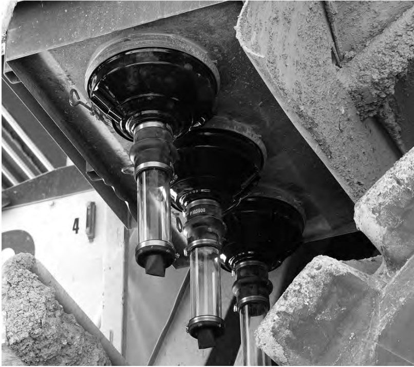
Dust Dumpa + PSD air cleaners extended the filter service life for a geothermal drill rig in Australia.
