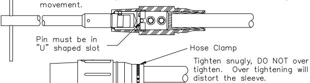
9. Wrap several layers of electrical tape over hose clamp to prevent accidental cutting of hands from sharp edges.
