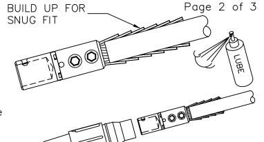
8. Connect Com-a—long  $\bigvee$  to contact and pull contact into sleeve. Pin on contact must line up with slot in sleeve. Rotate com-a—long while pulling if necessary to line up pin and slot.
