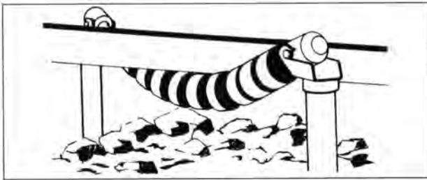
Figure 5 Poor housekeeping practices
