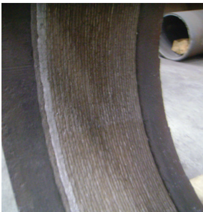
Flat ID pipe cladding with Stoodly CP-2000
