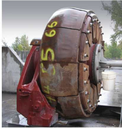
Segment roll repair with Stoodly 100HD
