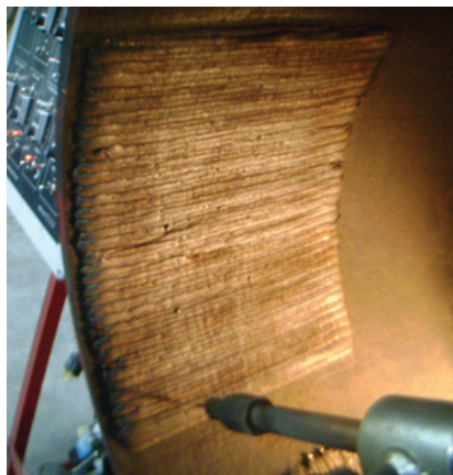
Horizontal ID pipe cladding with Stoodly CP-2000
