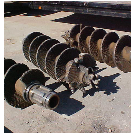
Auger repair with Stoodly 101HC
