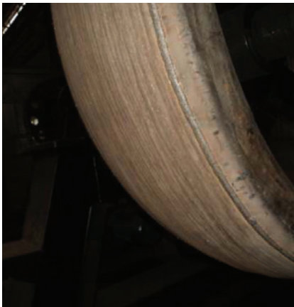
Crusher Roll Repair with Stoodly 100HD
