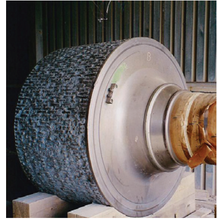
High pressure cement roll repaired with Theraclad Roll Build 3 and hardfaced with Stoodly 600
