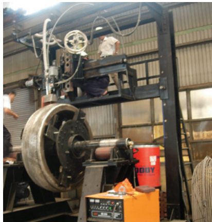
Crusher Roll Repair with Stoodly 100HC
