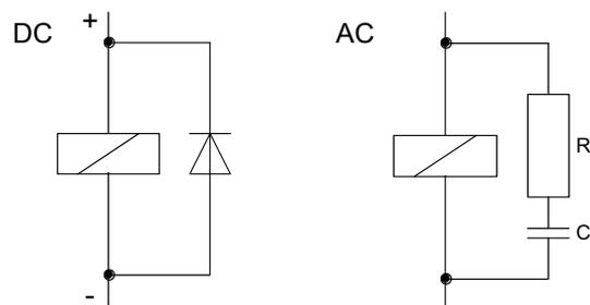
Fig. 23 Suppressor circuit DC/AC
