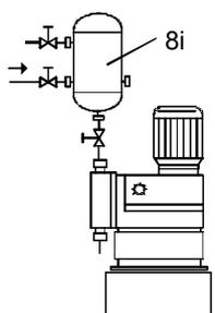
**Fig. 9** Installation with discharge-side pulsation damper
