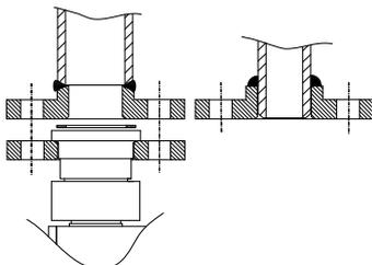
Fig. 15 Connection of DN 32 pipe lines
