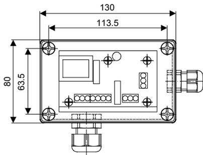
Fig. 21 Electronics enclosure
