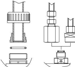
Fig. 14 Connection of DN 20 pipe lines
