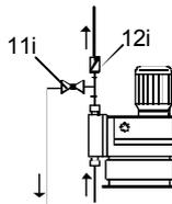
Fig. 5 Installation with ball valve and non-return valve
