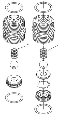
**Fig. 28** Stainless-steel or plastic valve DN 20,
