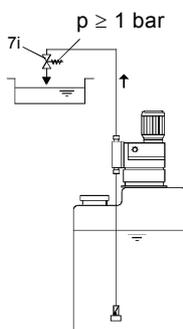
**Fig. 11** Installation with pressure-loading valve
