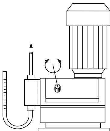
Fig. 20 Stroke-length adjustment
