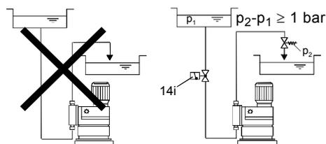
**Fig. 12** Installation to avoid the siphon effect
