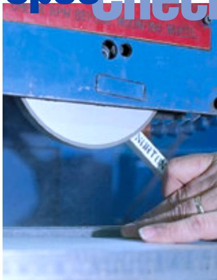
Selecting the appropriate dressing stick for each application depends on the wheel size, type, speed, specification and grit size, as well as the material being worked. Initial starting specifications are listed below. We recommend testing several sticks to find the best one for your application.
