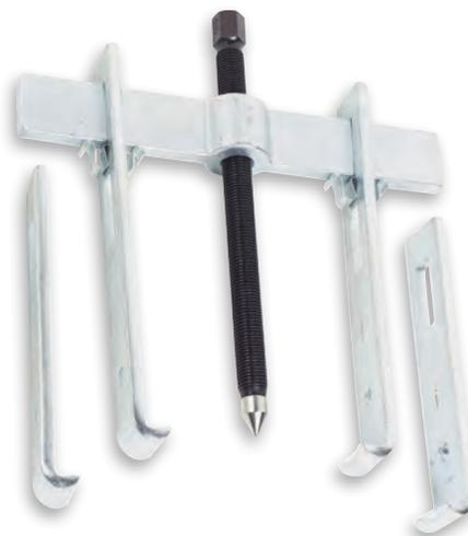
NOTE: Puller removes a gear with two sets of straight jaws, bolted together for extra reach. Set comes with two sets of jaws — Jaw No. J4015 has a 4-11/16" reach and No. J4016A has a 7-1/8" reach. Bolted together they easily clear the 8" long gear shaft.
