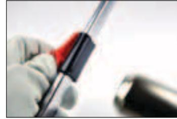
Using a standard heat gun, evenly heat the underside of the Shrink Loop while keeping the heat source approximately 1" (2.5 cm) away from the Shrink Loop. Avoid heating the care label.
