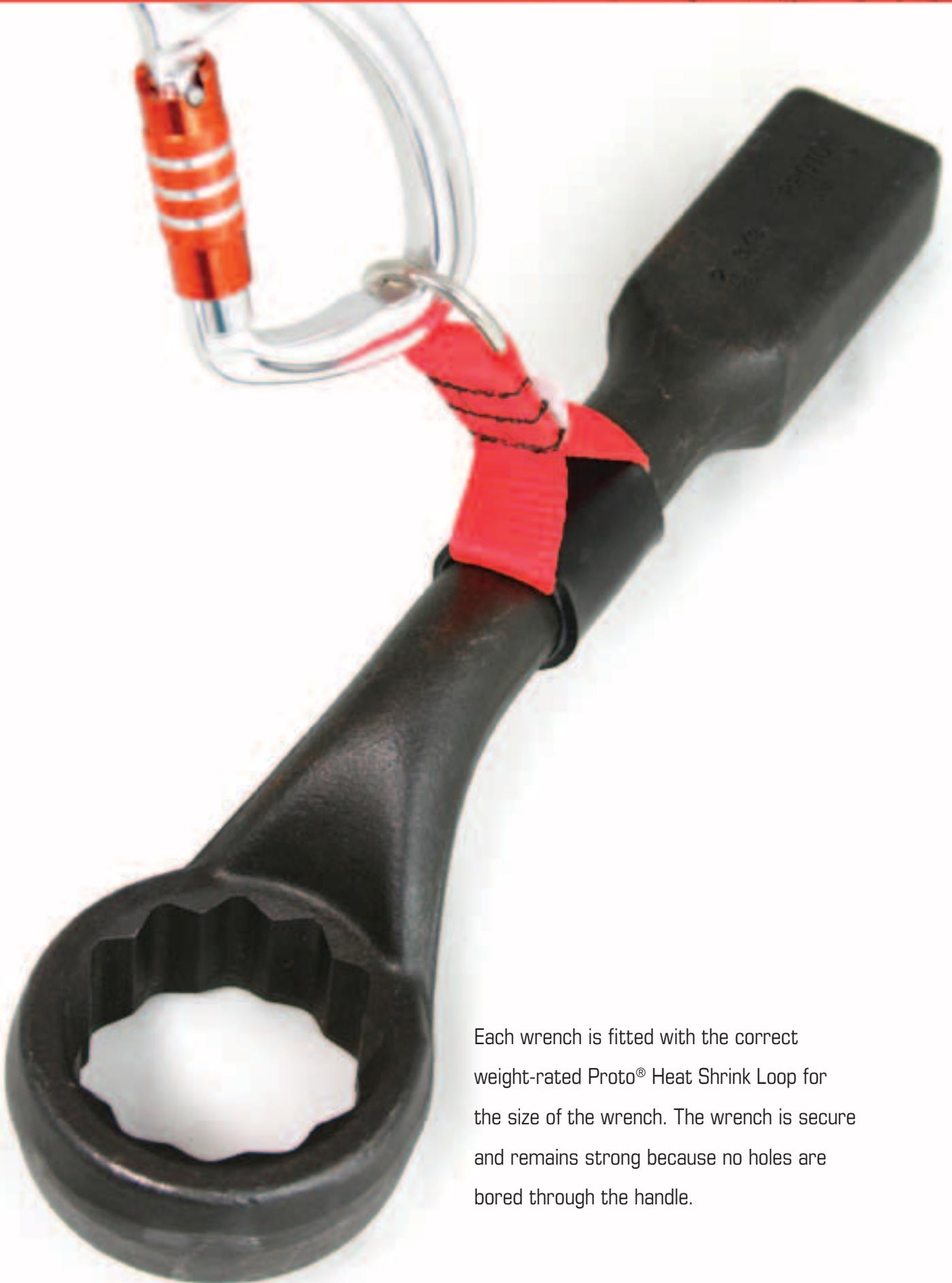
Each wrench is fitted with the correct weight-rated Proto® Heat Shrink Loop for the size of the wrench. The wrench is secure and remains strong because no holes are bored through the handle.
