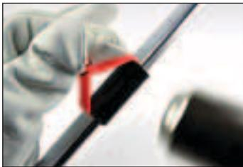
Heat the top section of the Shrink Loop.
