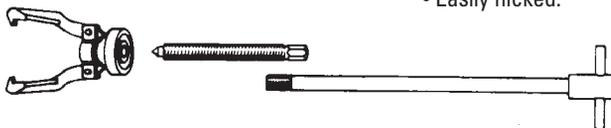
Switching from a Forcing Screw to a Slide Hammer used to be a problem. You had to unscrew with Forcing Screw from BOTH Crossblock and Adjusting Cone and this caused you to lose the set of your Jaws. Then you had to "hook-up" all over again. No More! Out comes the Screw and in goes the Slide Rod. You've got a Slide Hammer Puller. The Adjusting Cone? It stays put... on the Crossblock.
