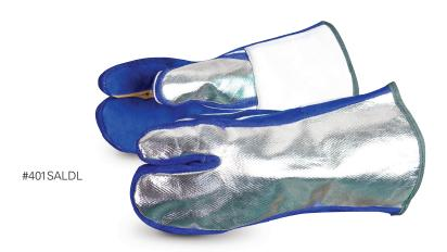
For maximum protection in high radiant-heat applications like Mig, Flux Core, Arc Air or Submerged Air welding. The aluminized back reflects up to 95% of radiant heat. The blue Tri-tan leather is resistant to ultra violet radiation. Cotton palm lined, wool lined back. Kevlar® sewn.
