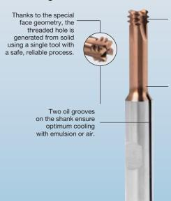
Thanks to the left cutting geometry the tool stabilizes itself during the climb milling process - perfect, true to gauge threads up to 66 HRC are guaranteed.
