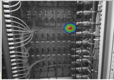
Did you know compressed air leaks often go unnoticed because the sounds blend in with other plant noises and can't be heard? Source Atlantic has invested in an acoustic imaging camera to help locate pressurized leaks that can cause increased energy bills, production inefficiencies and shorten the lifespan of equipment.
